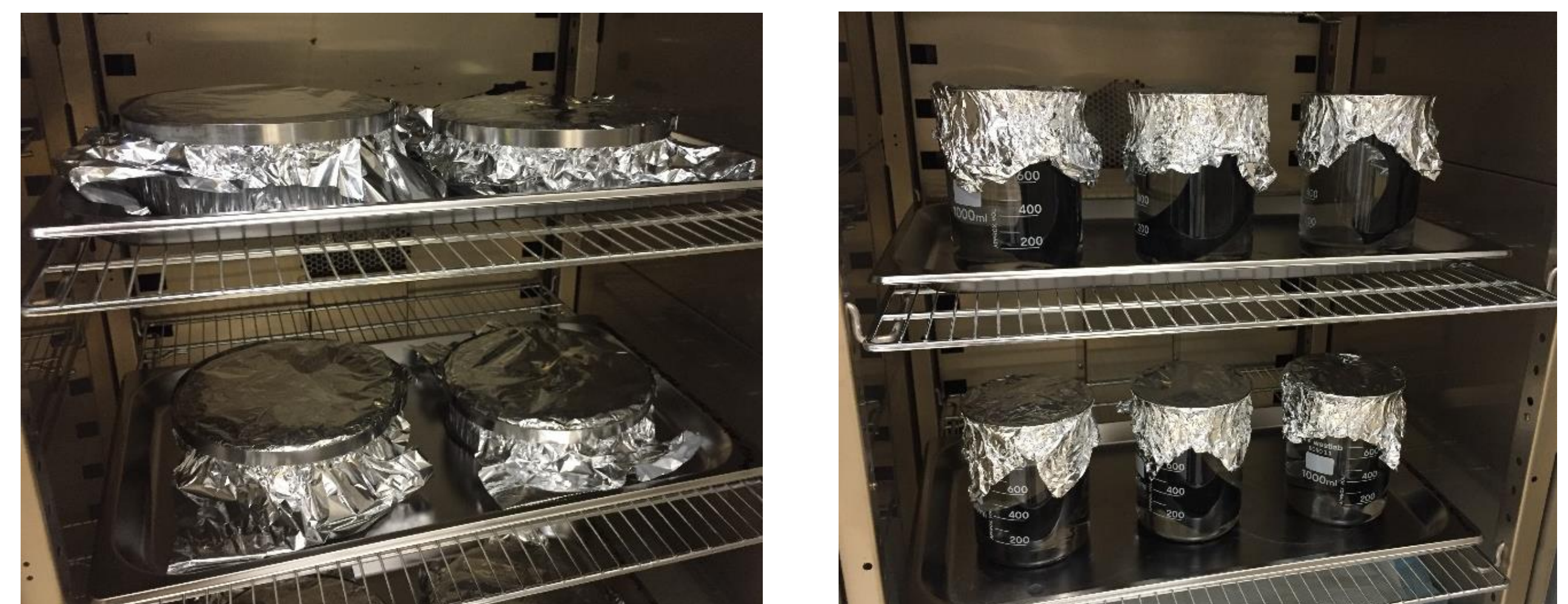
Figure 2: Stagnating pipe samples with the a) capped method, and b) static immersion method
